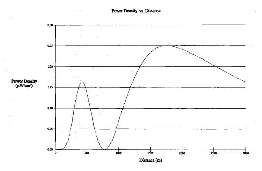
Effective Radiated Power = 30 kW Horizontal and Vertical Antenna Type = ERI Rototiller EPA Type Number of Bays = 4 Spacing Between Bays = .5 wavelengths Radiation Center above Ground = 450 meters
